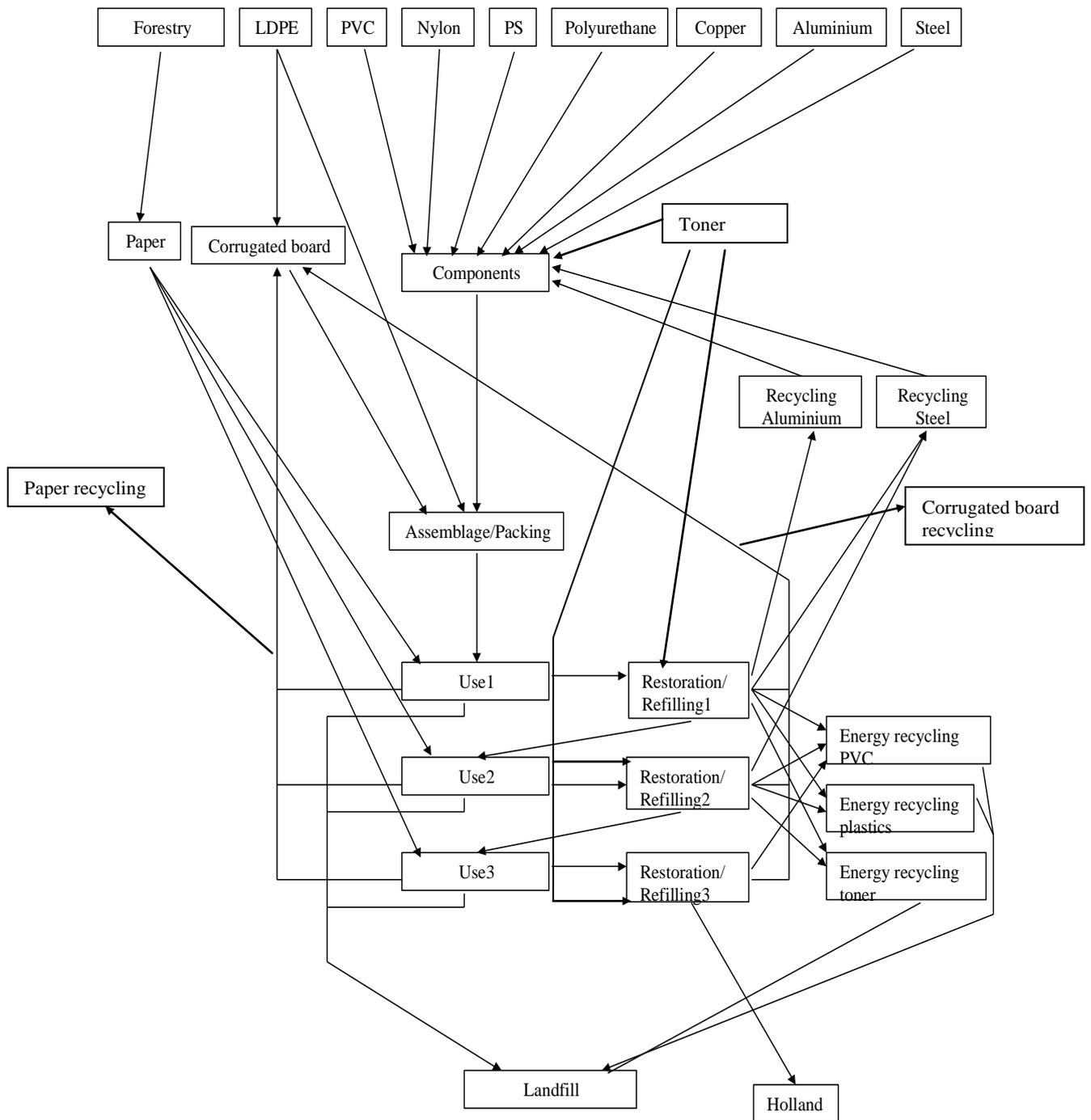
Figure 2. The life cycle of a re-used toner cartridge
