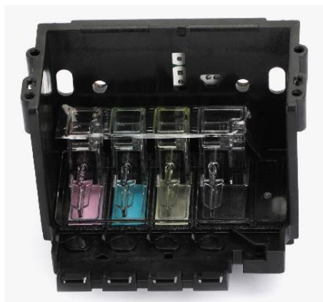
Figure 74. Example of printer with individual cartridges for each color
