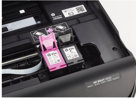
Figure 75. Example of printer with one cartridge for monochrome and another cartridge for the three colors
