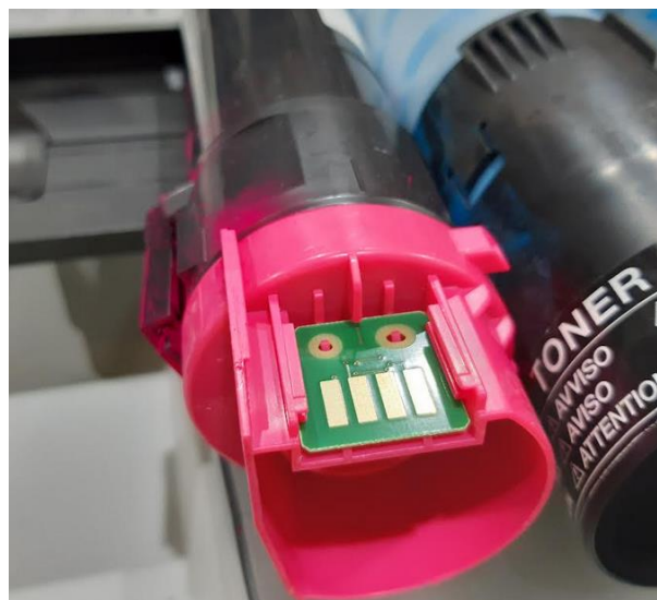
Figure 72. Chip in toner cartridge
